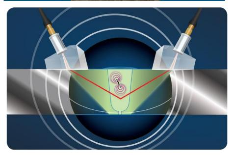
Time of Flight Diffraction (ToFD)
